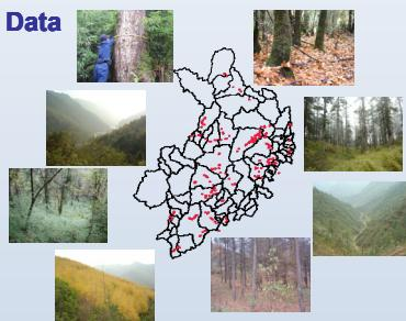
Ground truth points (red dots) acquired using real-time differentially corrected GPS receivers between 2007 and 2009 were used for calibration and validation of the land cover classification of remotely sensed data. Pictures show some landscape characteristics.
