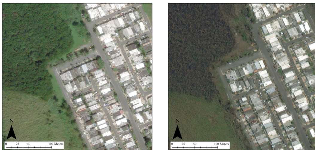
Fig. 9. Before and after damage detection for a mixed urban/vegetated area Puerto Rico. The MODIS based disturbance index had a value of 1.43, which increased to 2.98 after the storm. Green vegetation is visible on both images. However, the after image shows the disappearance of several trees in the urban area, as well as a browning of the forested region in the upper left. Note that the disturbance value before the storm was relatively high (1.43) as a result of the mixed nature of this pixel and a drought. Nevertheless, the disturbance index increased substantially as a result of the storm. (For interpretation of the references to colour in this figure legend, the reader is referred to the web version of this article.)
