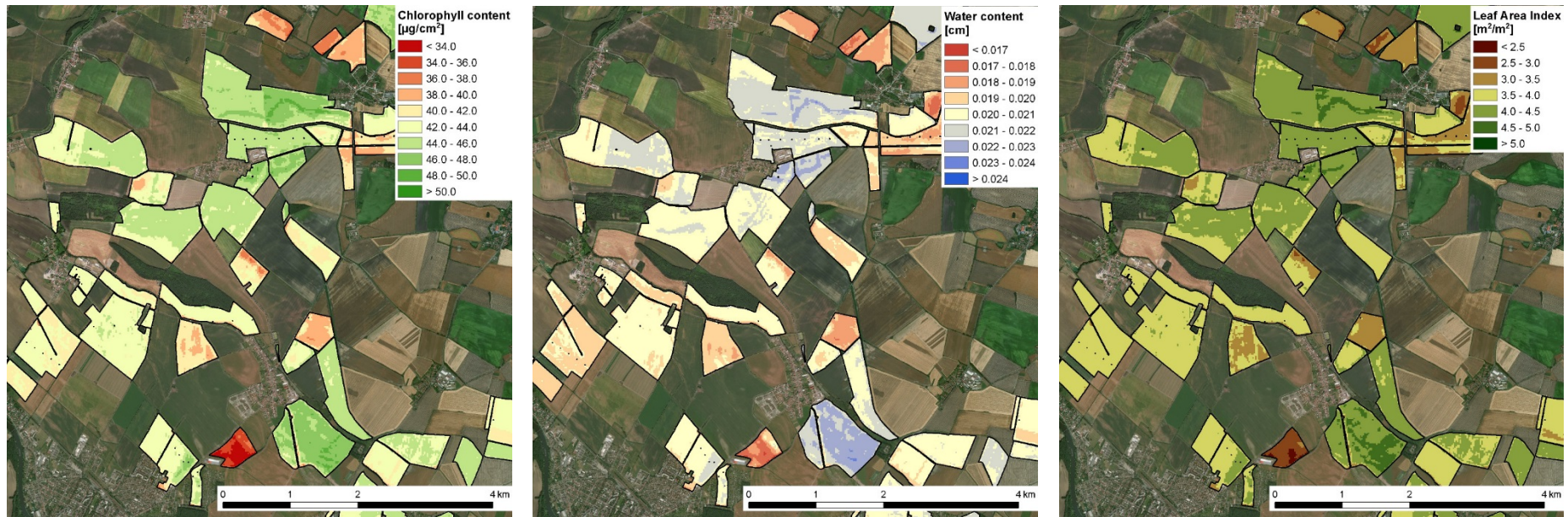
Example of the retrievals of leaf chlorophyll content (left), water content (middle) and leaf area index (right)
