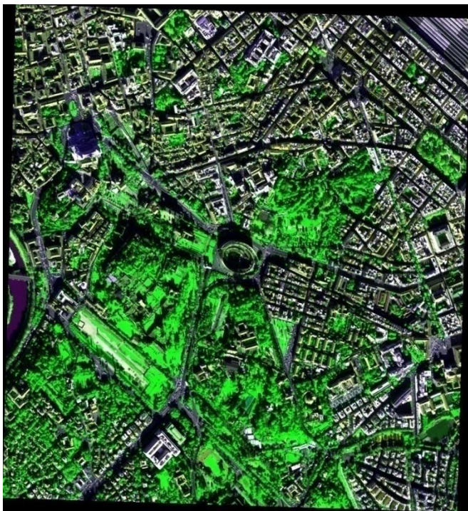
Fig. A. 8-band WorldView-2 VHR image of the city of Rome, Italy, acquired on 2009-12-10, at 10:30 a.m., depicted in false colors (R: band R, G: band NIR1; B: band B) (provided by DigitalGlobe, http://www.digitalglobe.com/index.php/70/Product+Samples ), calibrated into TOA reflectance. Spatial resolution: 2.0 m.
