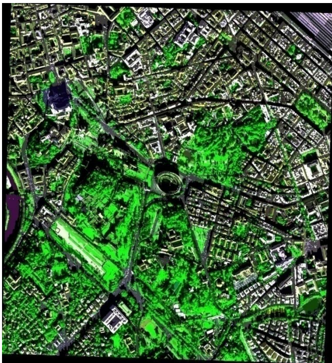
Fig. C. Segment-based piecewise constant approximation of the 8-band WorldView-2 VHR image of the city of Rome, Italy, acquired on 2009-12-10, at 10:30 a.m., depicted in Fig. A. Spatial resolution: 2.0 m. Note: the bridge has disappeared (Omission error!!!)
