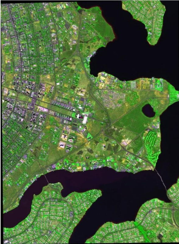
Fig. A. 8-band WorldView-2 VHR image of the city of Brazilia, Brazil, acquired on 2010-08-04, at 13:32 p.m., depicted in false colors (R: band R, G: band NIR1; B: band B) (provided by DigitalGlobe, 8-Band Challenge), calibrated into TOA reflectance. Spatial resolution: 2.0 m.
