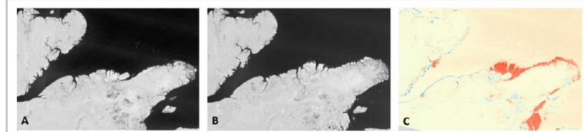
A. Amazon delta Aug. 2017 (before Belo Monte dam completion) and B. Amazon delta Aug. 2022 (after completion). C. Difference between 2017 and 2022. Red are areas where delta expanded and blue are areas where delta receded.
