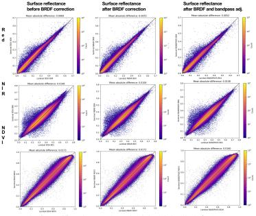
The reflectance difference between Landsat-8 and Sentinel-2A/B in the red band (1<sup>st</sup> row), NIR (2<sup>nd</sup> row), and NDVI (3<sup>rd</sup> row), after each of the processing steps: atmospheric correction (1<sup>st</sup> column), BRDF correction (2<sup>nd</sup> column), and bandpass adjustment (3<sup>rd</sup> column). The HLS processing has reduced the reflectance difference between the two sources.
